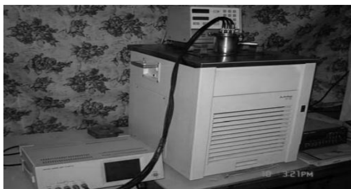
Figure 3: AC conductivity and dielectric measurement setup.
