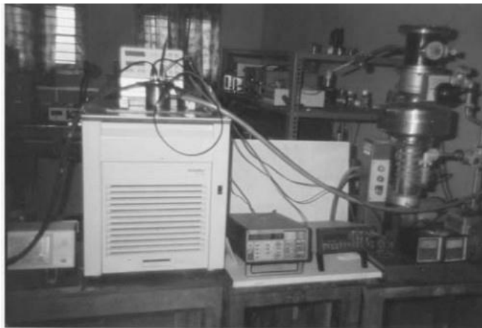
Figure 2: DC conductivity measurement setup.
