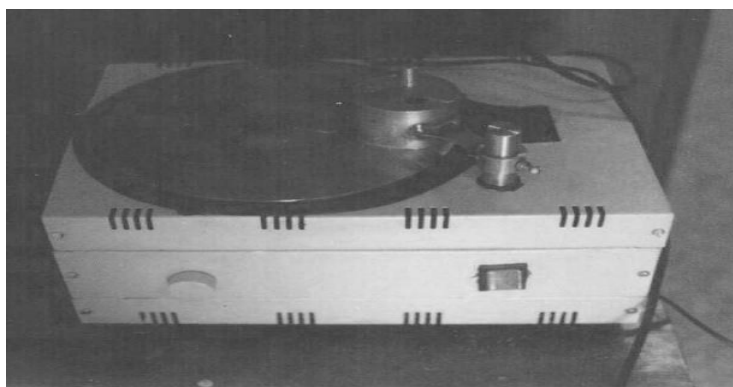
Photograph of the crystal polishing unit.
